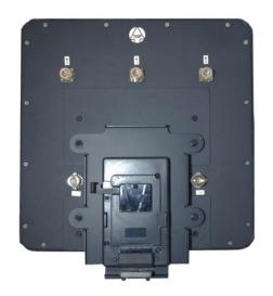
1) Panel antenna pre-installed V-mount bracket and 3/8" to 1/4" screw mount adapter rear view
