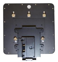
1) Panel antenna pre-installed G-mount bracket and 3/8" to 1/4" screw mount adapter rear view
